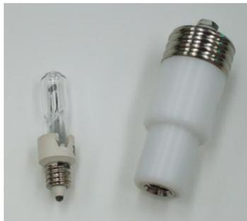
Total spectral radiant flux standard lamps (75 W halogen) issued from NIST (300 to 1100 nm)
