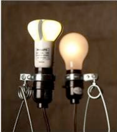
Figure 2. Philips's LED-based A Lamp Incandescent Replacement ("L-Prize" Entry)
